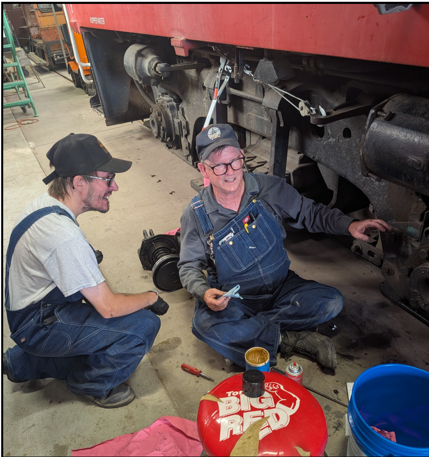
Tim Wamsley, assisted by Justin Hyland, is working on a leaking air cylinder on SP #3873. This is routine maintenance for our volunteers at Campo.
